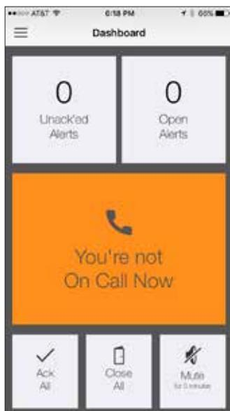
The SCADA-as-a-service system that Harris County Water Control and Improvement District No. 1 installed enables alarms and notifications to be delivered via email, voice message, and text message, as well as with a smartphone app like the one pictured. Ops Genie
