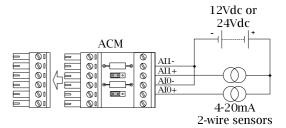
Note: very high precision resistors should be used for all of these applications, e.g. 0.01%, 5ppm.
