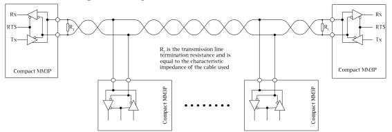
The standard RS485 receiver input impedance, called a unit load, is  $12K\Omega$ ; a standard RS485 driver can drive up to 32 such loads. The Compact MM3P RS485 transceivers present an eighth of this unit load (96K $\Omega$ ) which allows up to 256 Compact MM3Ps on a RS485 communication link.
